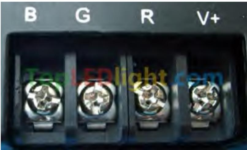
Adopt four sheath wires as connecting wires ,meanwhile,black wire→ + brown wire→R yellow wire→G blue wire→B
